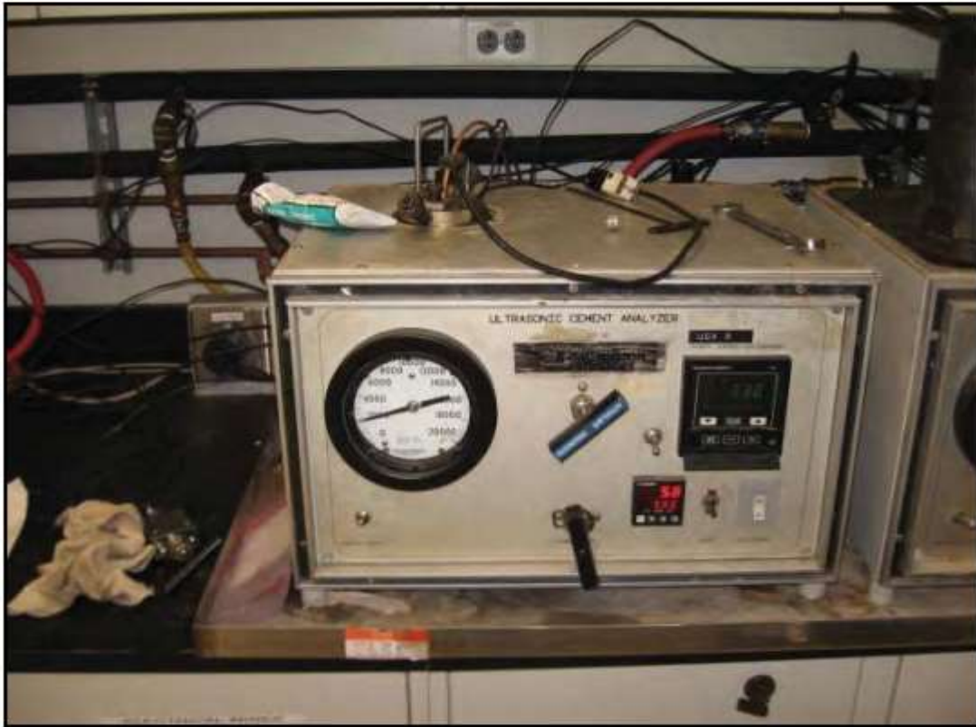
Figure 1: Ultrasonic Cement Analyzer for Compressive Strength Testing Source: (API, 2006)
